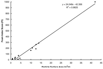
Figure 2. Foam Index Score as a function of particle surface area.
