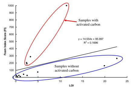
Figure 1. Foam Index Score as a function of LOI in fly ash samples.
