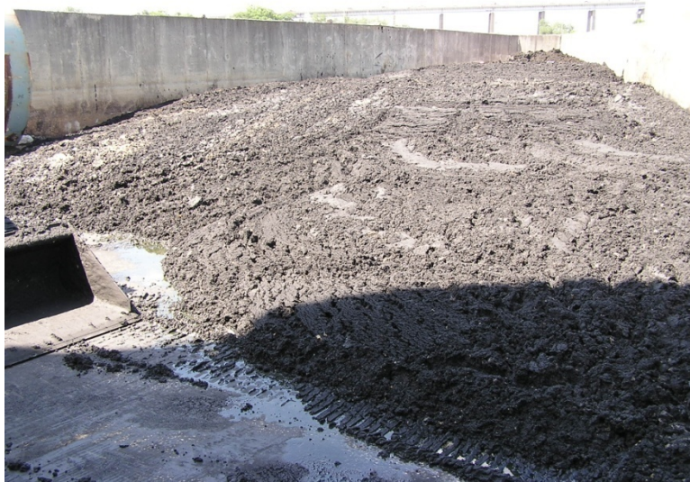
Figure 7. Treated sludge stockpiled for curing prior to disposal
