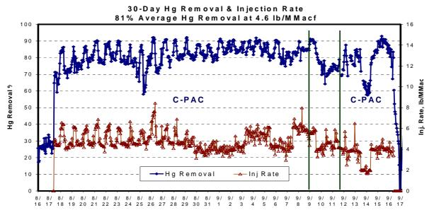
Figure 1. Crawford Unit 7 Mercury Removal & Injection Rates Over 30 Days.
