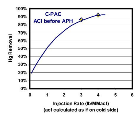
Figure 4. Mercury Removal Rate of C-PAC at Waukegan.
