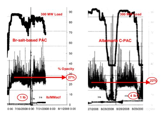
Figure 5. Stack opacity with load with the injection of different sorbents.
