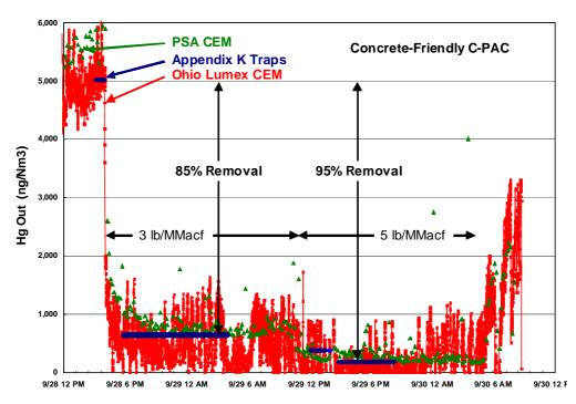
Figure 3. Mercury Removal & C-PAC Injection rate at Corette.
