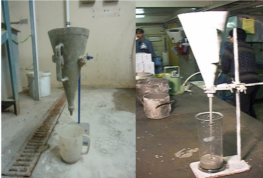
Fig 4.1 Comparison of flowability in foamed concrete regarding the self-weight effect (left hand image is 200 kg/m 3 , right hand image 300 kg/m 3 ; both at 0.5 w/c ratio).
