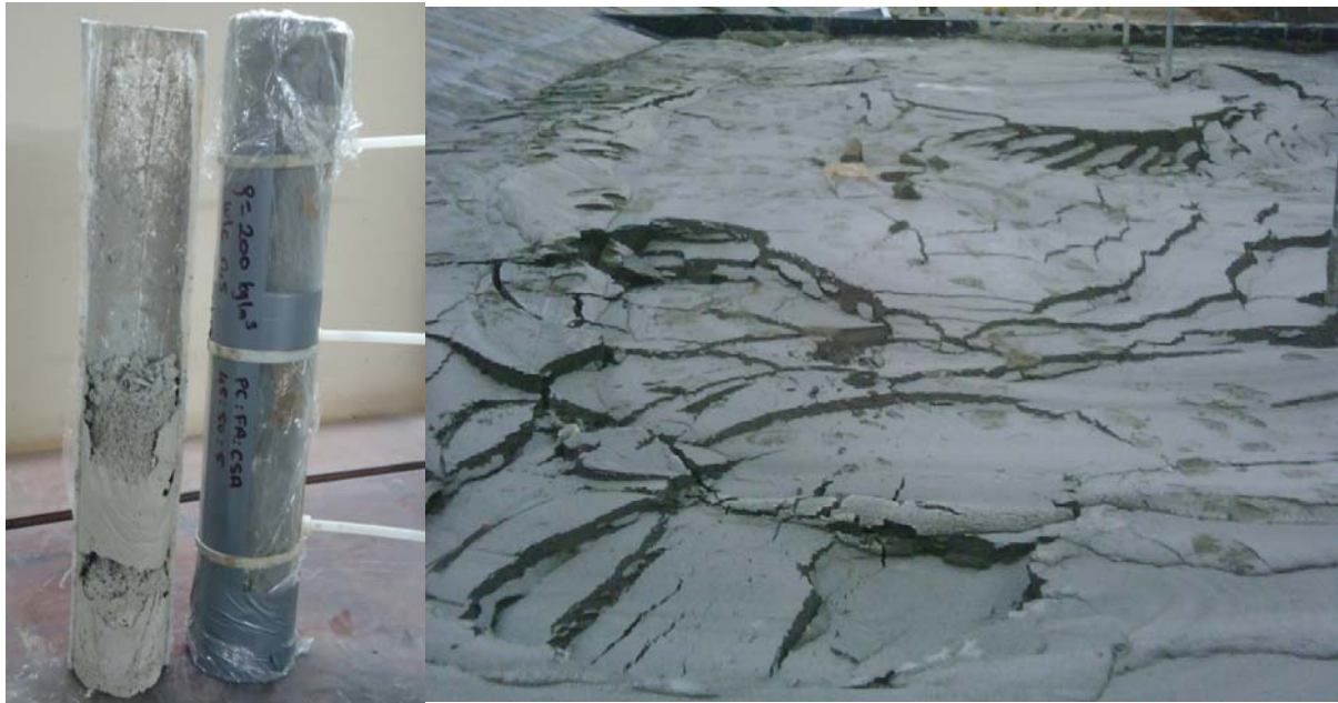
Fig 2.1 Example of instability in the laboratory (left) and in practice (right; courtesy of Propump Engineering Ltd., 2009)
