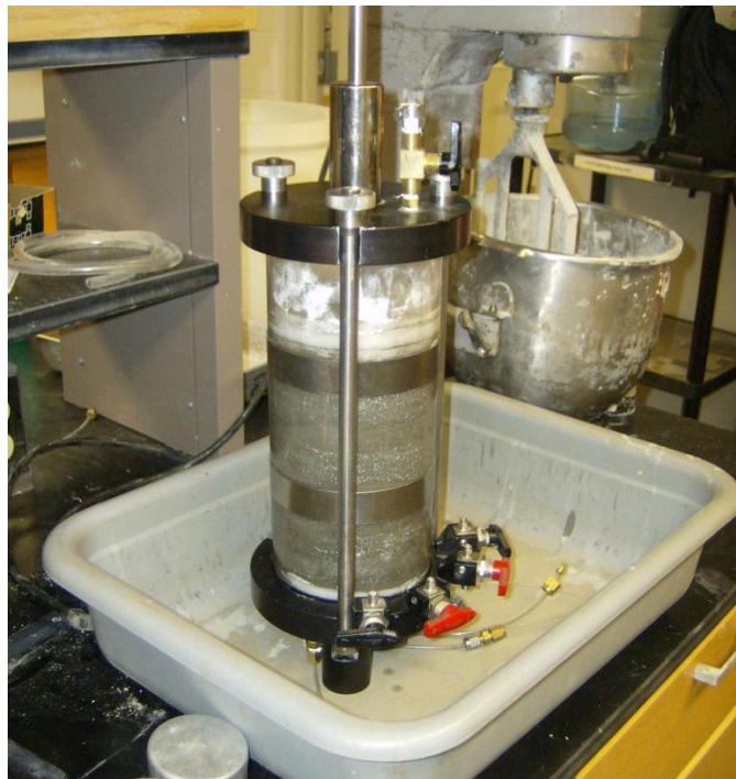
Figure 1. Modified Triaxial Chamber for Preparation of Pluviated Samples
