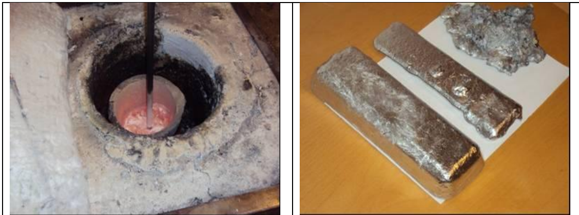
Fig. 1. Left: Molten alloy stirring (pre-heated FA particles are added to the melt in the rate of 3g/min). Right: A356 Al/KFA 10% wt. composites.
