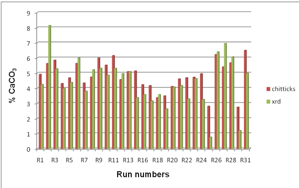
Figure 7: Correlation of mass % CaCO 3 yield determined by quantitative XRD and Chittick test.
