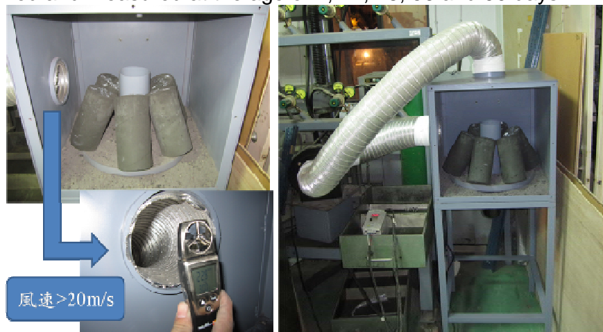
Figure 2 Erosion test of wind with coal ash particles
