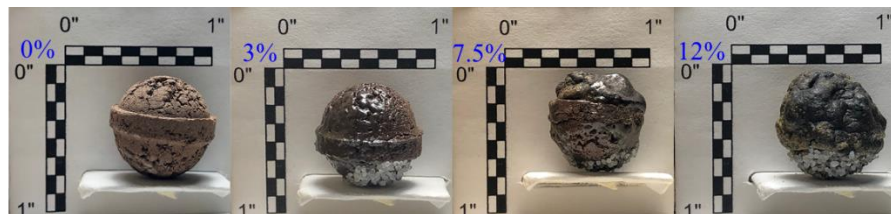
184 185 186 Figure 5. Front views of sintered FA4 at 1160 °C for 8 min (NaOH concentration is indicated on 187 the upper left corner)
