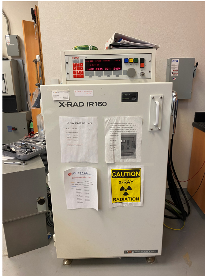
Figure 2.5: A photo of the X-RAD iR-160 compact cabinet industrial X-ray irradiation system. The cabinet X-ray system consists of XRP generator (control unit, power supply, and high-voltage (HV) tank), cabinet, and water cooler.
