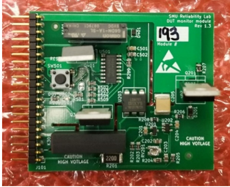
Figure 4.6: A picture of the current sensing module. Total power consumption at 600 V is approximately 0.9 W. The low-cost modular design allows for fast replacement in the event of damage. The circuit was designed and validated by Danyal Ahsanullah.
