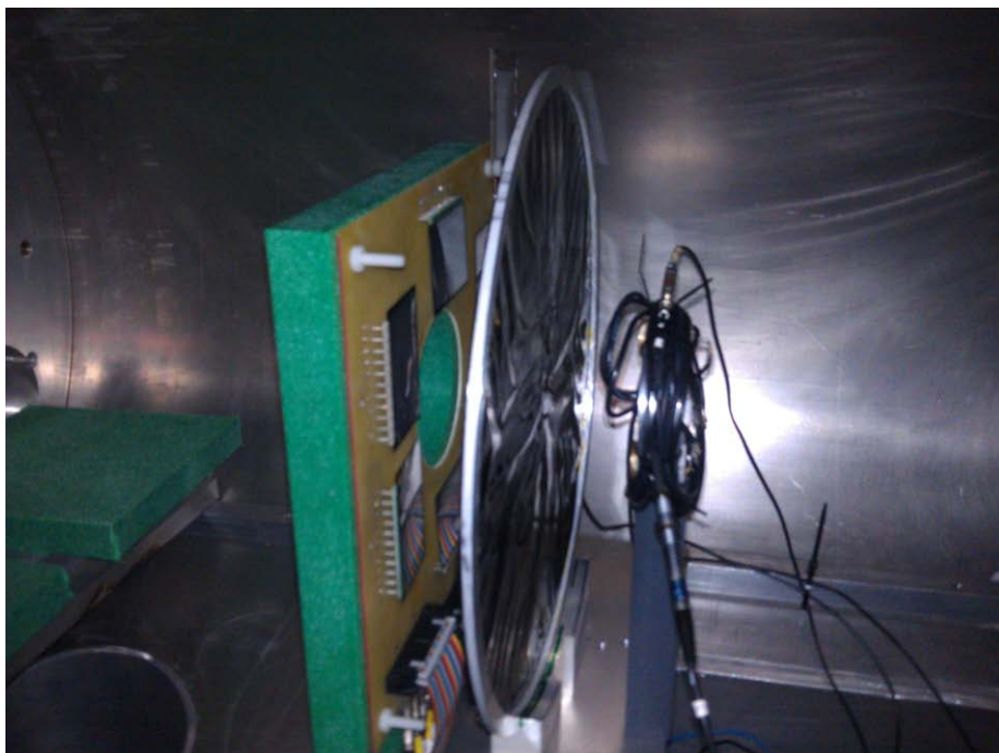
FIG. 1. Picture of the experimental setup as placed in the reaction chamber. 6 seven strips silicon detectors (Micron Semiconductors design I, thickness 300\ \mu\text{m} ) are placed after the target position, facing the catcher foil. The catcher is a polypropylene layer of thickness 7.5\ \mu\text{m} placed at 3 cm from the silicon detectors. The catcher has a central hole to allow the beam to pass through and three additional holes in correspondence of the position of the monitor detectors. A Faraday cup is placed at the end of the line at about 5 m from the target. Two different ^{232}\text{Th} targets were placed in the target ladder: one of thickness 11\ \text{mg}/\text{cm}^2 and another of thickness 6.3\ \text{mg}/\text{cm}^2 followed by a ^{12}\text{C} degrader of thickness 3\ \text{mg}/\text{cm}^2 .
