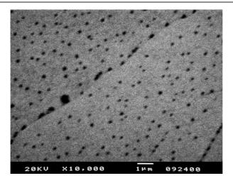
Figure 5. SEM image of a freshly cut CdI<sub>2</sub>–Cd<sub>i</sub> surface.
