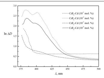
Figure 1. The difference absorption spectra of non-stoichiometric  $CdI_2$  crystals at T = 290 K.
