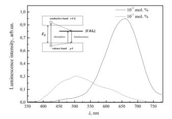
Figure 2. Cathodoluminescence of  $CdI_2$  crystals with different  $Cd_i$  concentrations at 290 K. The inset shows the scheme of electronic transitions which cause the additional absorption and emission bands connected with non-stoichiometric cadmium.
