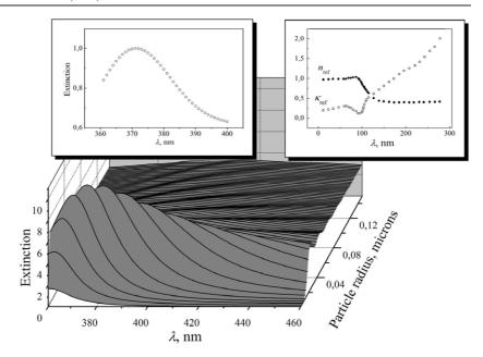
**Figure 6.** Panoramic extinction spectra of cadmium iodide crystals with cadmium clusters calculated in the frame of Mie theory. The inset on the right shows the refractive index dispersion (according to [26]). The inset on the left illustrates the calculated extinction spectrum, which represents the averaged contribution of the clusters observed in the crystals with  $10^{-1}$  mol%  $Cd_i$  concentration.
