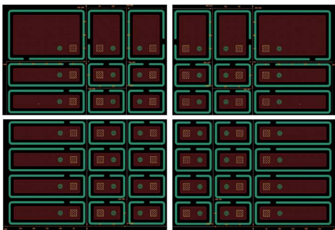
Fig. 3. The detailed design of a forward pixel sensor at the four corners of each ROC. In green are the p-stop rings around the pixel implants.
