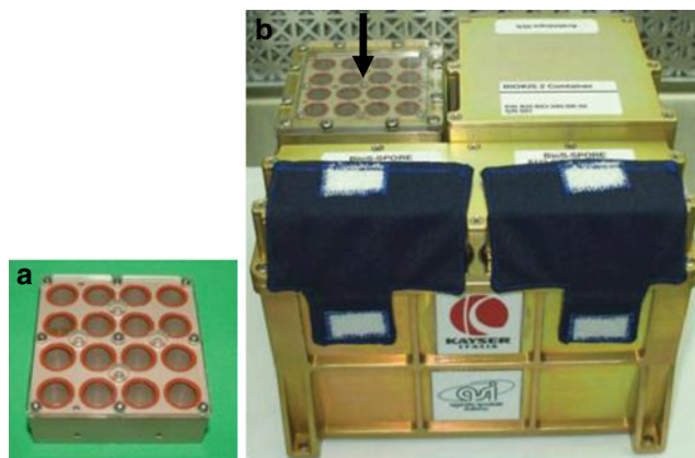
Fig. 6 a PHOTOEVOLUTION EU. b Black arrow indicates EU integrated on top of the BIODON 002
