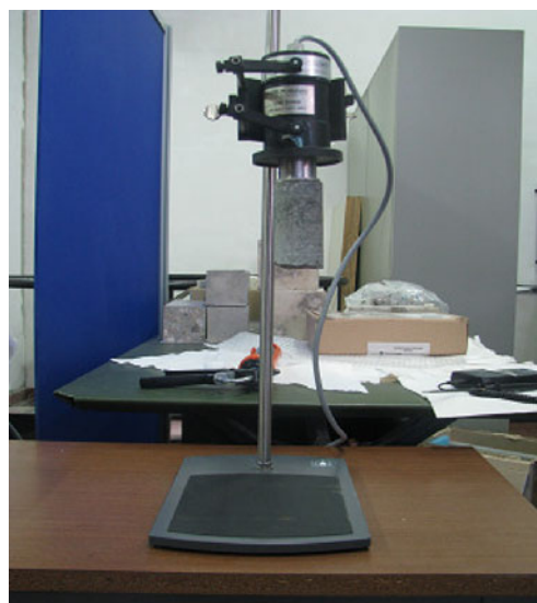
Fig. 7 The Luserna stone specimen connected to the ultrasonic horn. The ultrasonic apparatus (Bandelin HD 2200) consists of a generator that converts electrical energy to 20 kHz ultrasound, and of a transducer that switches this energy into mechanical longitudinal vibration of the same frequency
