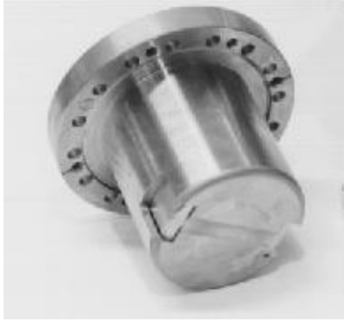
Fig. 11. Picture of a Roman pot made at CERN. This conventional design is taken as a baseline for the new Roman pots at the LHC
