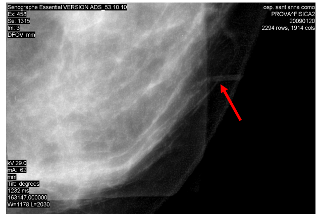
Fig. 5 Mammogram of the prototype depicted in Fig. 4 on an anthropomorphic breast phantom. The image was taken with an Essential Senographe (GE Healthcare, USA [9]) in maximum contrast mode. The exit of the fiber (see arrow) can be identified while the embedded part of the fiber is not visible in this Mammogram.
