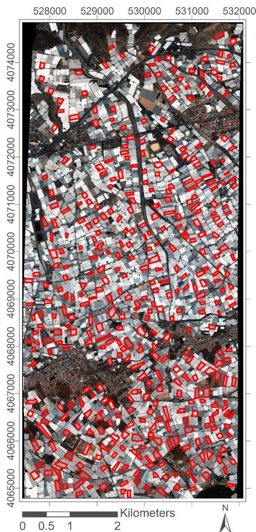
Figure 2. 400 reference geometries manually digitized (polygons in red) representing PCG on the WV3 PANSH RGB orthoimage.
