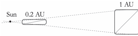
Figure 1. Initial and final domains of simulation (and plasma volume) in the ecliptic plane. Thin lines: direction of mean magnetic field. For all runs, the aspect ratio of the domain varies from 1/5 to unity. In the figure, the mean magnetic field angle with the radial varies from \tan^{-1}(1/5) \simeq 11.3^\circ to \tan^{-1}(1) = \pi/4 .
