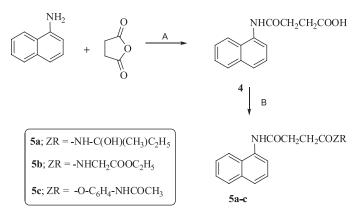
Scheme 2. Reagents and conditions: (A) Acetic acid, stirring at rt, (B) ethyl chloroformate/triethylamine, at 10 °C then H-ZR and stirring at rt.
