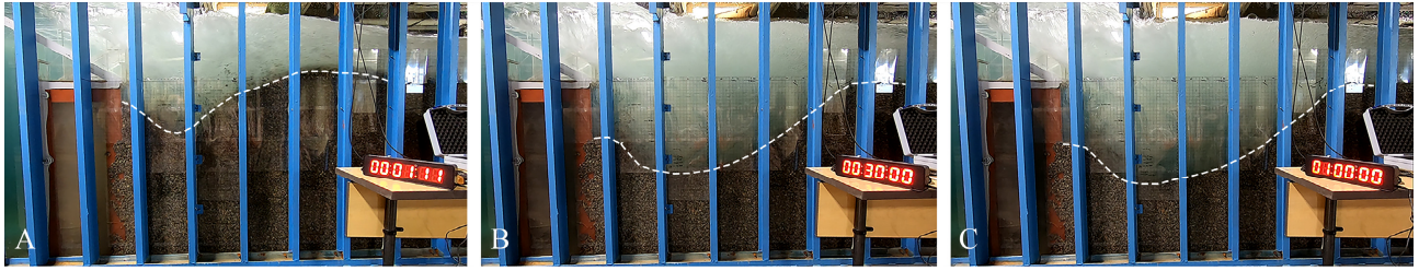
Fig. 6. Scour development with time for (A) Initial Phase, (B) Second Phase, and (C) Final Phase.
