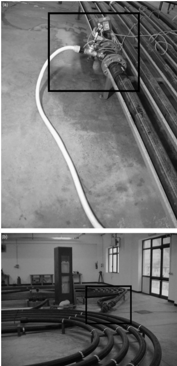
Figure 4 | Connection between the main pipe and the branch: (a) RPLBV system and (b) RHDPEBV system. In the square the connection node is highlighted.
