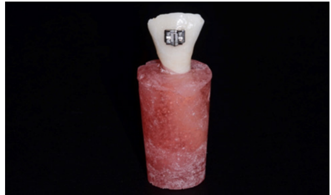
Figure 4 Cow mandibular incisor with a bracket bonded directly.
