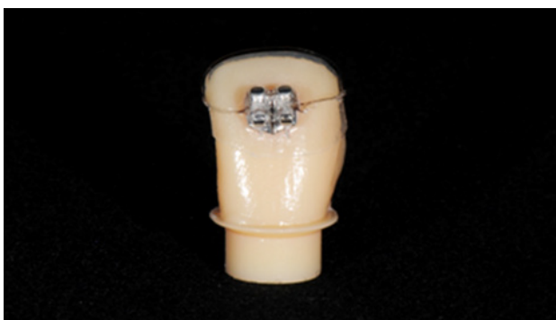
Figure 6 Resin replica with bracket and two thermo-formed trays.
