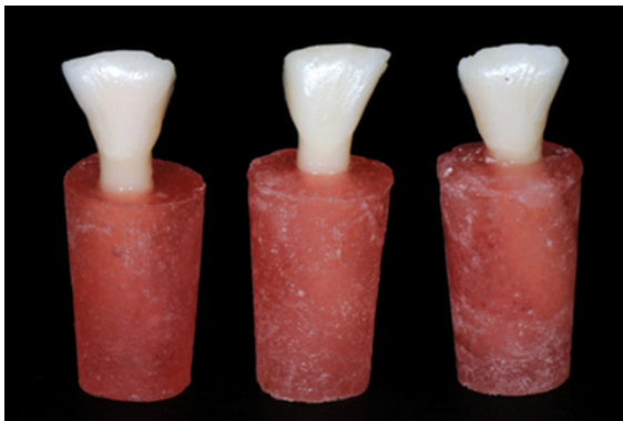
Figure 2 Teeth individually secured in cold resin (Leocryl; Leone, Sesto Fiorentino, Italy).
