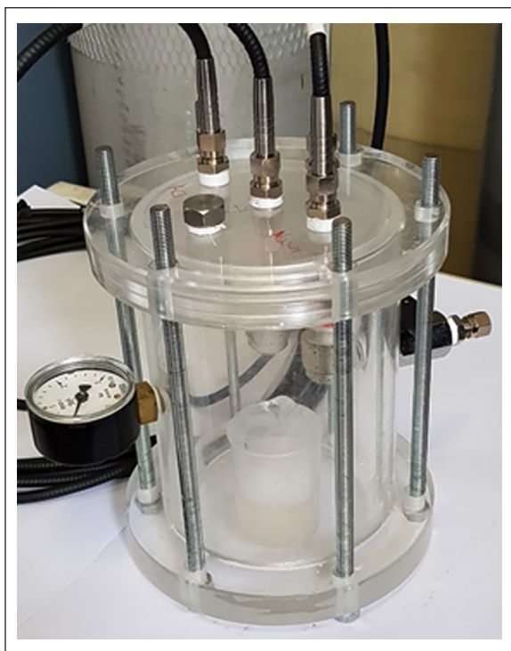
Figure 3. Set up for the pH measurement with fiber optic sensors.
