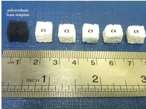
Fig. 1: Prepared composite samples using polyurethane foam template.
