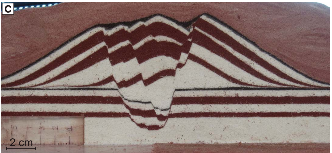
Figure 15. Vertical cross sections of a deformed analogue cone cut perpendicular to the basal shear. Cross sections progress from cuts on the basement (A) toward the summit of the cone (C).
