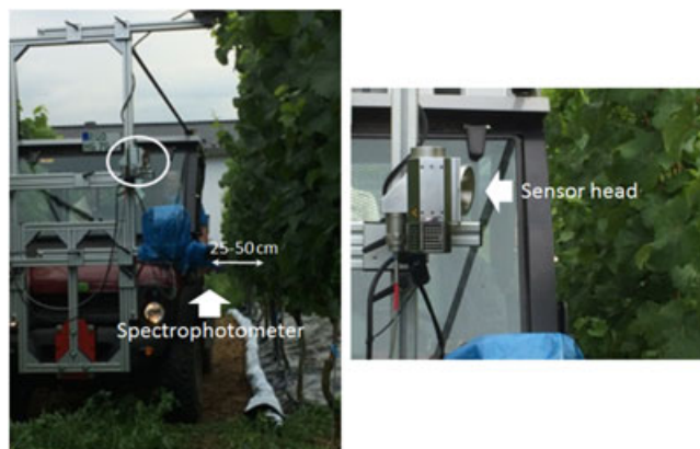
Figure 1. Illustration of the set-up of the near infrared system operating from the moving all-terrain vehicle.
