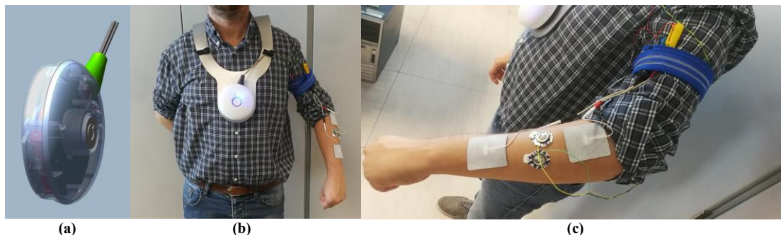
Fig. 6. (a) 3D plot of the FITFES including internal electronics, (b) photograph of the final device, (c) an example of electrode placement of FITFES for treating a left hemiplegic hand: both EMG (circular shape) and stimulating (square shape) electrodes are on the wrist/finger extensor muscles.
