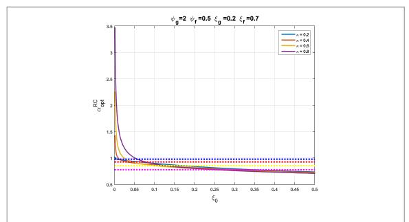
Figure 7. Optimal value of  $\alpha$  assuming white noise (dotted lines) and filtered white noise (continuous lines) for different damping ratios; Spectral configuration (c).
