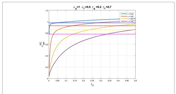
Figure 6. Optimal value of  $\alpha$  assuming white noise (dotted lines) and filtered white noise (continuous lines) for different damping ratios; Spectral configuration (b).
