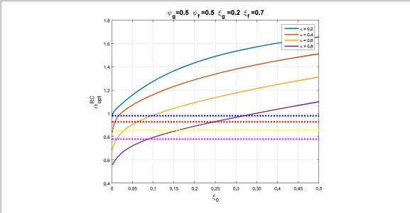
Figure 5. Optimal value of  $\alpha$  assuming white noise (dotted lines) and filtered white noise (continuous lines) for different damping ratios; Spectral configuration (a).
