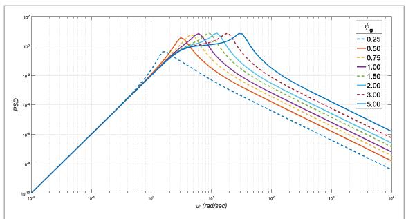
Figure 3. Clough Penzien spectra for different values of frequency ratio  $\psi_g$ . The main system period is assumed as 1 s ( $\omega_0=2\pi \, ({\rm rad/\, sec})$ ) while  $\psi_p=0.5$  and  $\xi_g=0.2$  and  $\xi_p=0.7$ .
