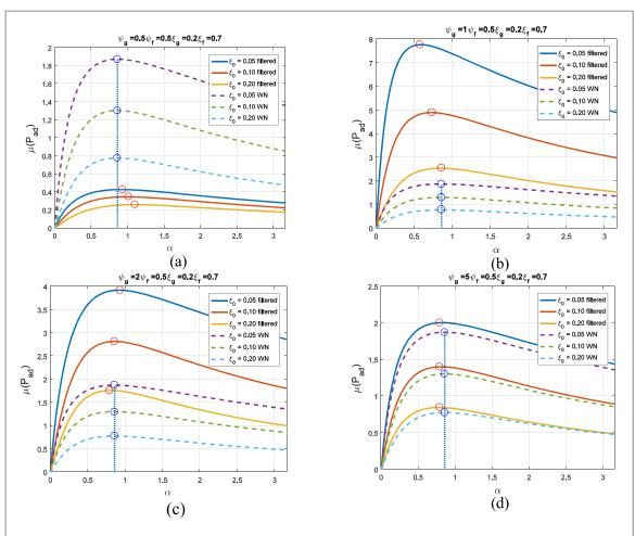
**Figure 4.** Energy efficiency assuming white noise (dotted lines) and filtered white noise (continuous lines) for different damping ratios and for different filter configurations. Maxima are reported with blue circles (white noise) and red circles (filtered input).
