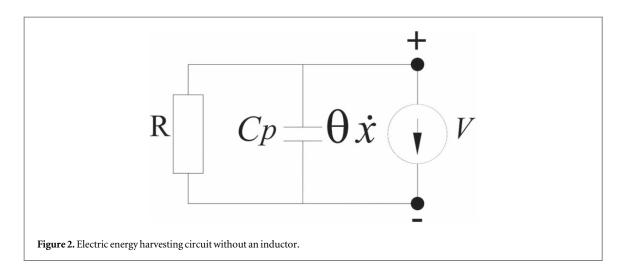
$\vartheta$  as  $v_{pz} = \theta \dot{x}$ ; and finally  $C_p$  is the capacitance of the piezoelectric element (Adhikari *et al* 2009, Erturk and Inman 2011, Adhikari *et al* 2016).
