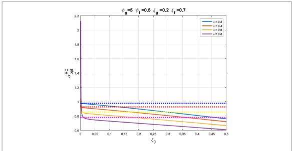
Figure 8. Optimal value of  $\alpha$  assuming white noise (dotted lines) and filtered white noise (continuous lines) for different damping ratios; Spectral configuration (d).
