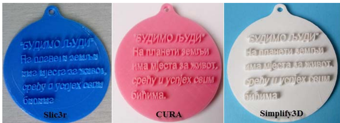
Figure 7. Photograph of the pendants manufactured by printing from three different slicer tools: Slic3r , Cura and Simplify3D .
