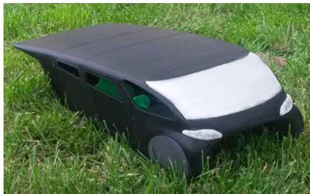
Figure 1. RP in-scale model of a Solar Car [30].
