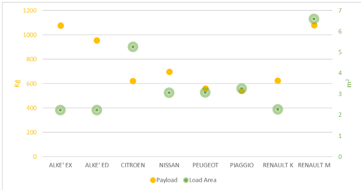
Fig. 4. Payload and load area. Positioning of the main Electric LCVs sold in the italian market (category N1).
