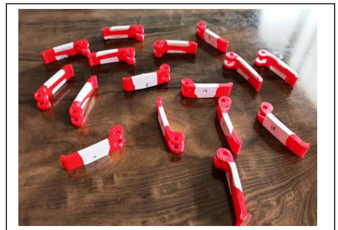
Fig. 2. Cam Levers Manufactured by FDM
