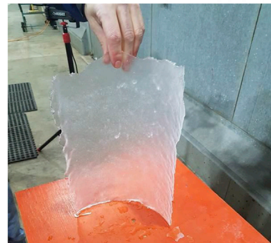
(b) Ice shell detached from a cable model in the NRC Climatic Testing Facility.
