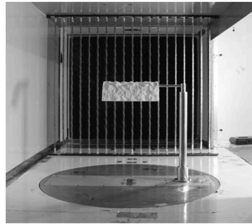
(b) Setup in the tunnel showing the S9-Sim model,
