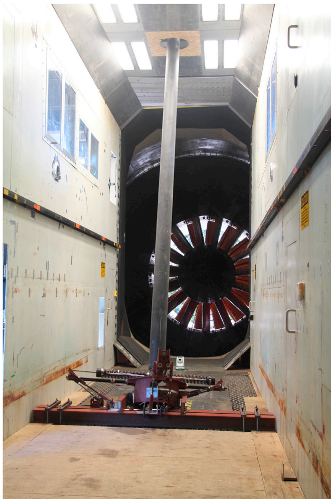
Fig. 3. Smooth cable model in the NRC 3 m × 6 m Wind Tunnel, looking upstream.
