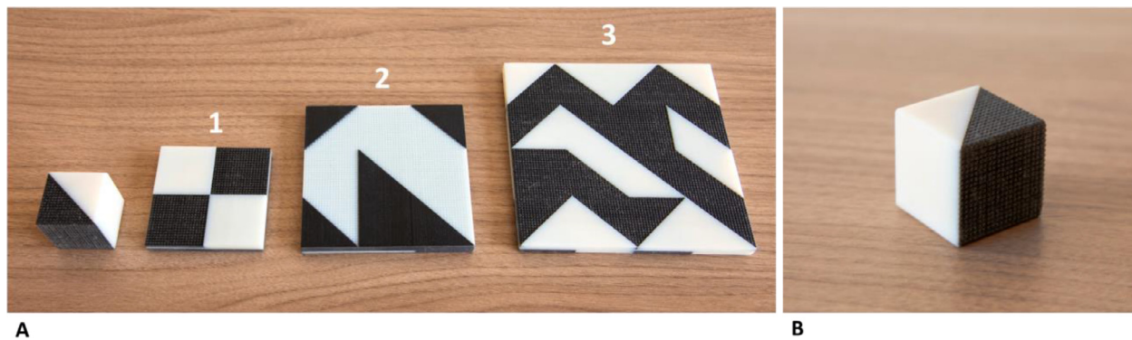
Fig. 1. Images of the test material. (A) Example of the three dimensions of the haptic designs. In relation to the size of the haptic block on the left edge of the image, 4 blocks are needed to compose haptic design 1, 9 blocks to compose haptic design 2 and 16 blocks to compose haptic design 3. (B) One of the 16 identical haptic blocks. In the picture, the faces of the cube that differ for color and texture are shown. Two faces of the cube are white with a smooth texture, two faces are black with a rough texture, and two faces are half black with a rough texture and half white with a smooth texture.
