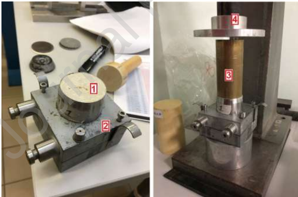
Figure 6 – Specimen of two-component grout before demoulding (left) and insertion phase of the specimen in the shear box (right). Sample held in the mould (1), Casagrande shear box (2), push cylinder (3), and pushing frame (4).
