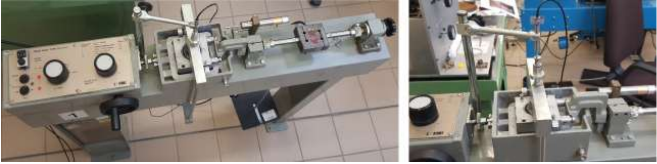
Figure 4 – Shear machine (left) and Casagrande shear box fixed on the shear machine (right).
