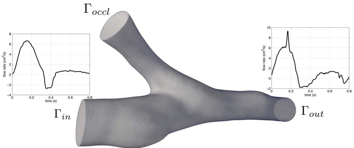
Fig. 7. Femoropopliteal bypass geometry. Graph of the inlet and outlet flow rates, as measured in [36].
