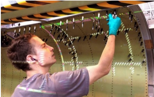
Fig. 6. AR projection systems used at Dassault Aviation (source: [15]).
