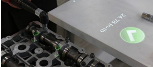
Fig. 5. Assembly instructions projected on the workbench and on the parts (source: [14]).
