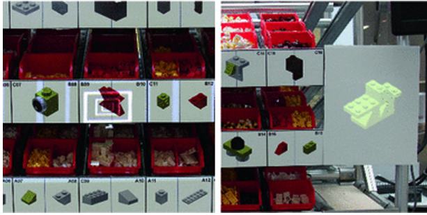
Fig. 7. Presentation of picking information and assembly instruction on a projection-based AR assembly station (source: [16]).
