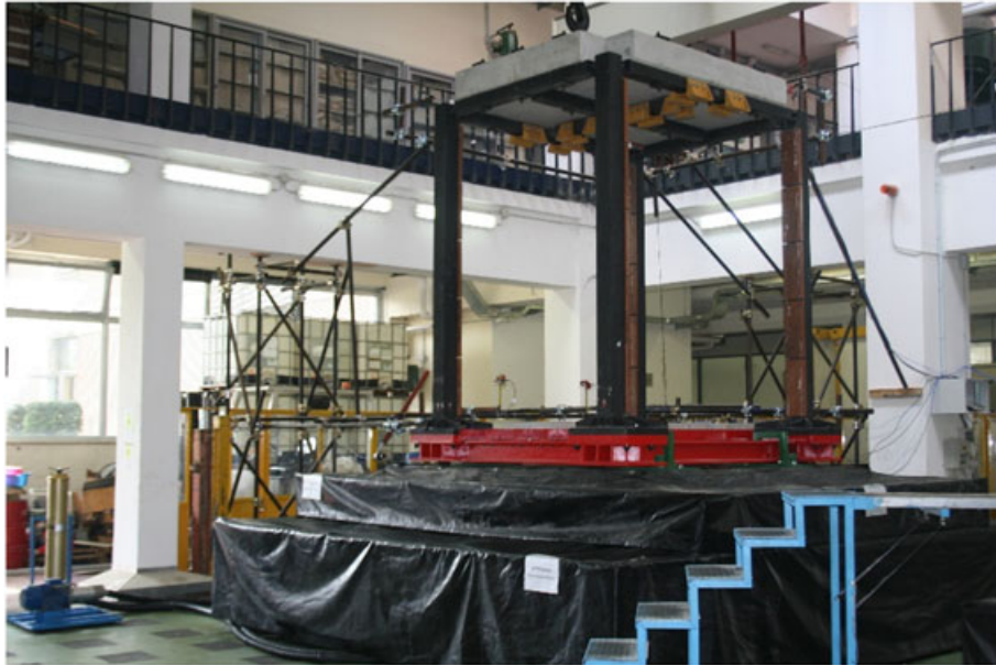
FIGURE 9 Tested isolated building
