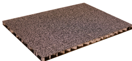
FIGURE 2 Aluminum sandwich with the speckle pattern
