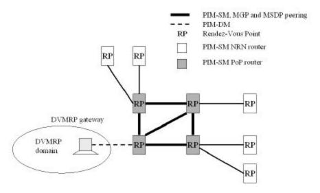
Figure 2. Logical model of present European multicast network
