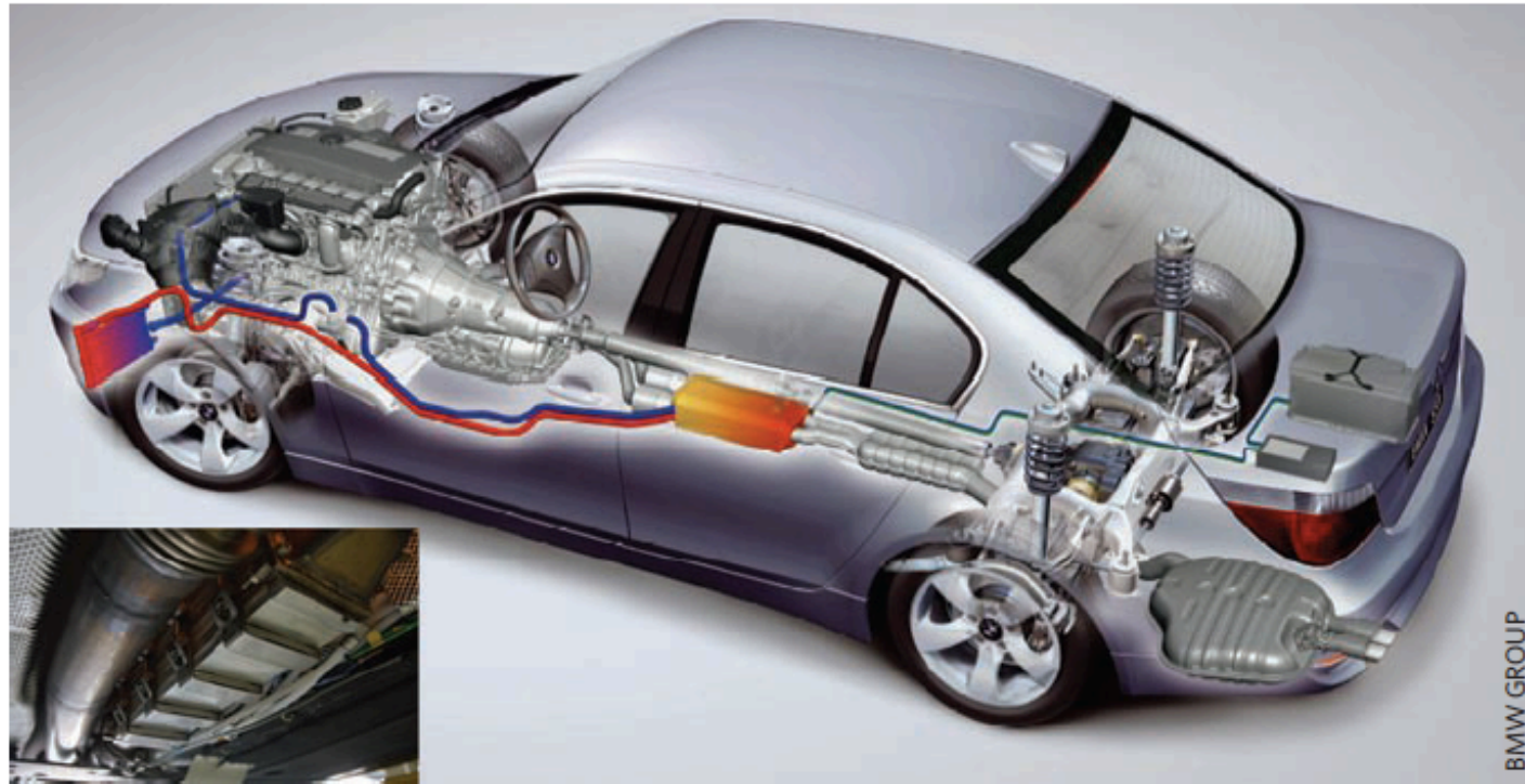
Figure 1 | Integrating thermoelectrics into vehicles for improved fuel efficiency. Shown is a BMW 530i concept car with a thermoelectric generator (yellow; and inset) and radiator (red/blue).
