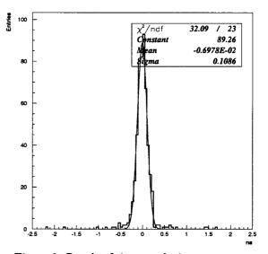
Figure 3. Result of time resolution measurements on a counter of the S1 layer.
