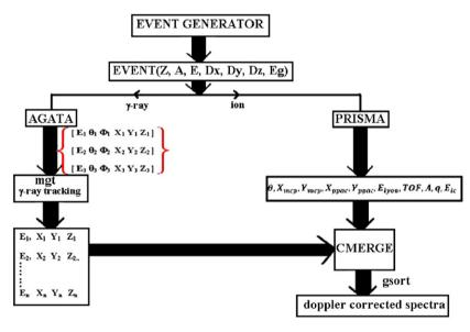
Fig. 2. Scheme of AGATA Demonstrator+PRISMA simulation.
