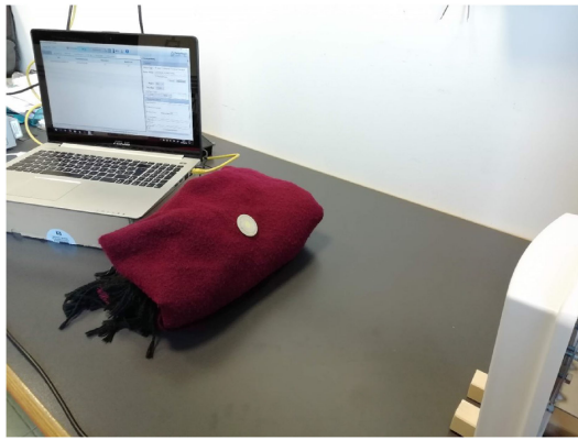
FIGURE 7. Test of the UHF transponder. The tag is interrogated with the Thing-Magic Nano - RAIN RFID reader in a realistic environment.
