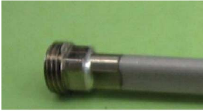
Fig. 9. The end part of an aluminum tube soldered to a nickel plated fitting.
