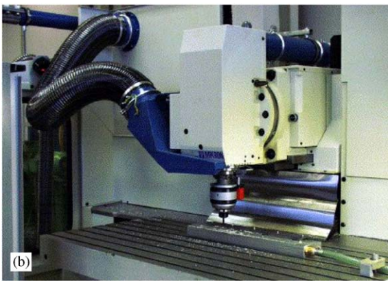
Fig. 6. (a) C–C impregnation chamber and (b) high speed milling machine.
