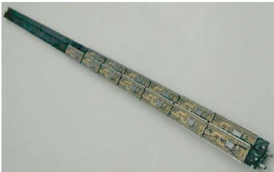
Fig. 3. Bi-stave assembly with dummy modules.
