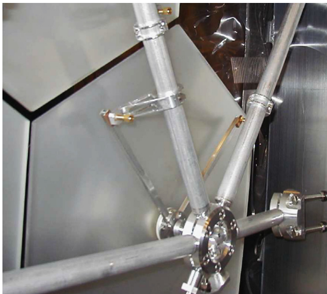
Fig. 1. Mirror wall rear face, detailed view: the mechanical arrangement for the angular adjustment of an individual mirror element is visible.
