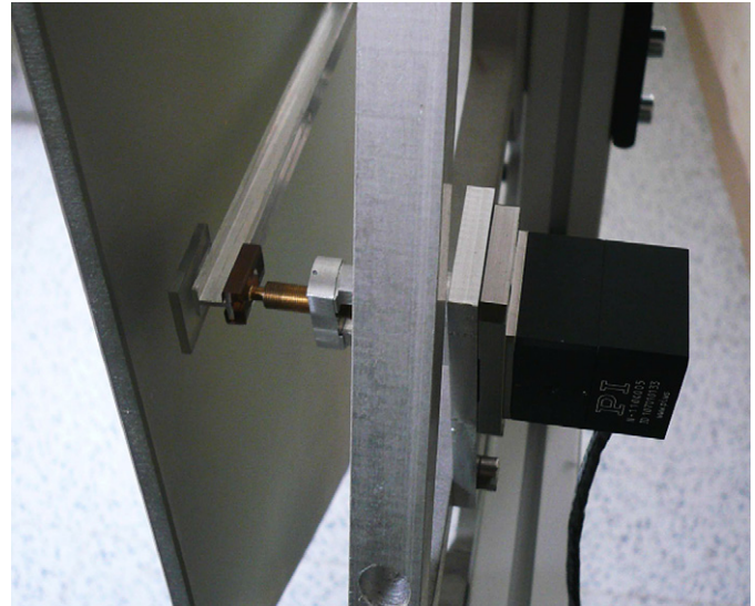
Fig. 3. Laboratory setup, the mirror rear side: the piezo actuator replaces one of the micrometric screws.
