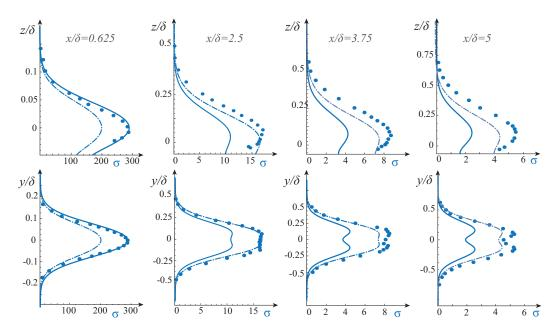
FIG. 8. Standard deviation for the LLS3. The points are the experimental values; the solid and dash-dot lines come from Eq. (8), with  $\tau_m^{(c)}$  and  $\tau_m^{(x)}$ , respectively.
