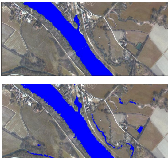
Figure 10. At the top, the water class before refinement, in the lower part the water class after refinement.
