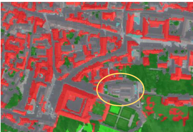
Figure 16. Same area after the classification with Random trees algorithm with an example of incorrect classification.
