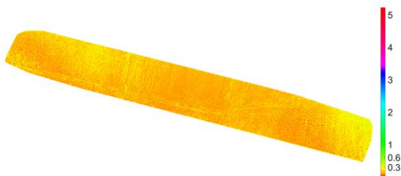
Figure 19. The cloud 3D distance maps after the ICP registration, between Blocks 3 and 4 in the overlapping area, expressed in meters
