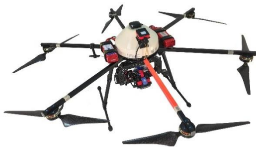
Figure 1. The HEXA-PRO UAV used for the survey equipped with the Parrot Sequoia camera
