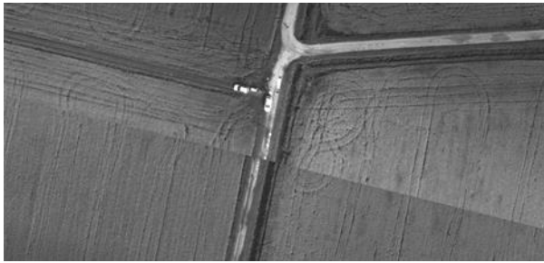
Figure 3. An excerpt of the green orthophoto in the overlapping area; a significant planimetric displacement is evident
